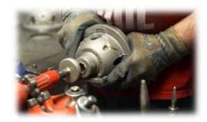
There is no dressing of the wheel required, as the grits are more fully exposed than in conventional wheels. And, because the wheel does not wear like a conventional wheel would, there is no loss of form or peripheral speed and less dust generated.
