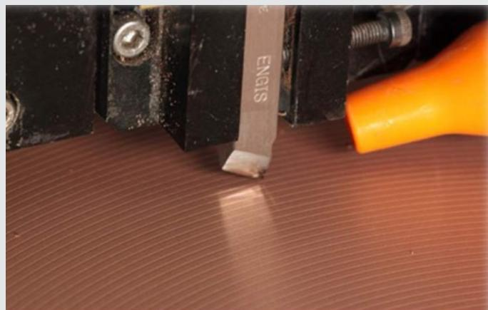
By incorporating a single point turning tool, as opposed to conditioning rings or similar tools which require operator skill in their accurate positioning, the overall lapping environment is rendered controlled and predictable.
