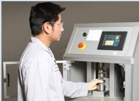
Engis has developed many innovations, including this patented apparatus for close monitoring of the crushing strength and fracture characteristics of finished diamond powder.
