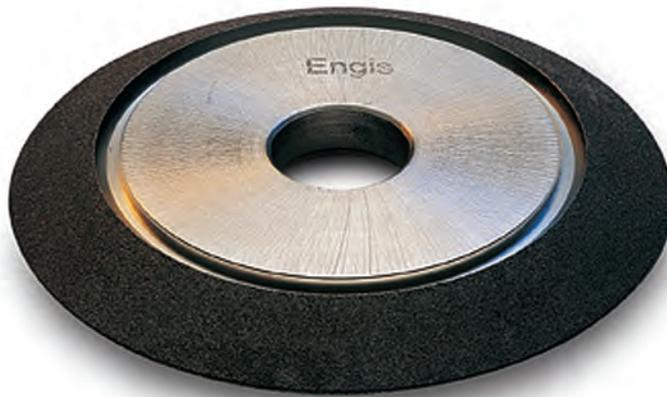
CBN plated grinding wheels...a highly productive alternative to aluminum oxide wheels for the sharpening of broach gullets. These wheels can be used on your conventional broach grinder without modification, however, for best results, equipment of rigid construction with a good spindle should be used. While wheel life is best when coolant is used, the operation can be done dry. The aggressive, free-cutting CBN superabrasive generates little heat. This is especially important in dry grinding.
