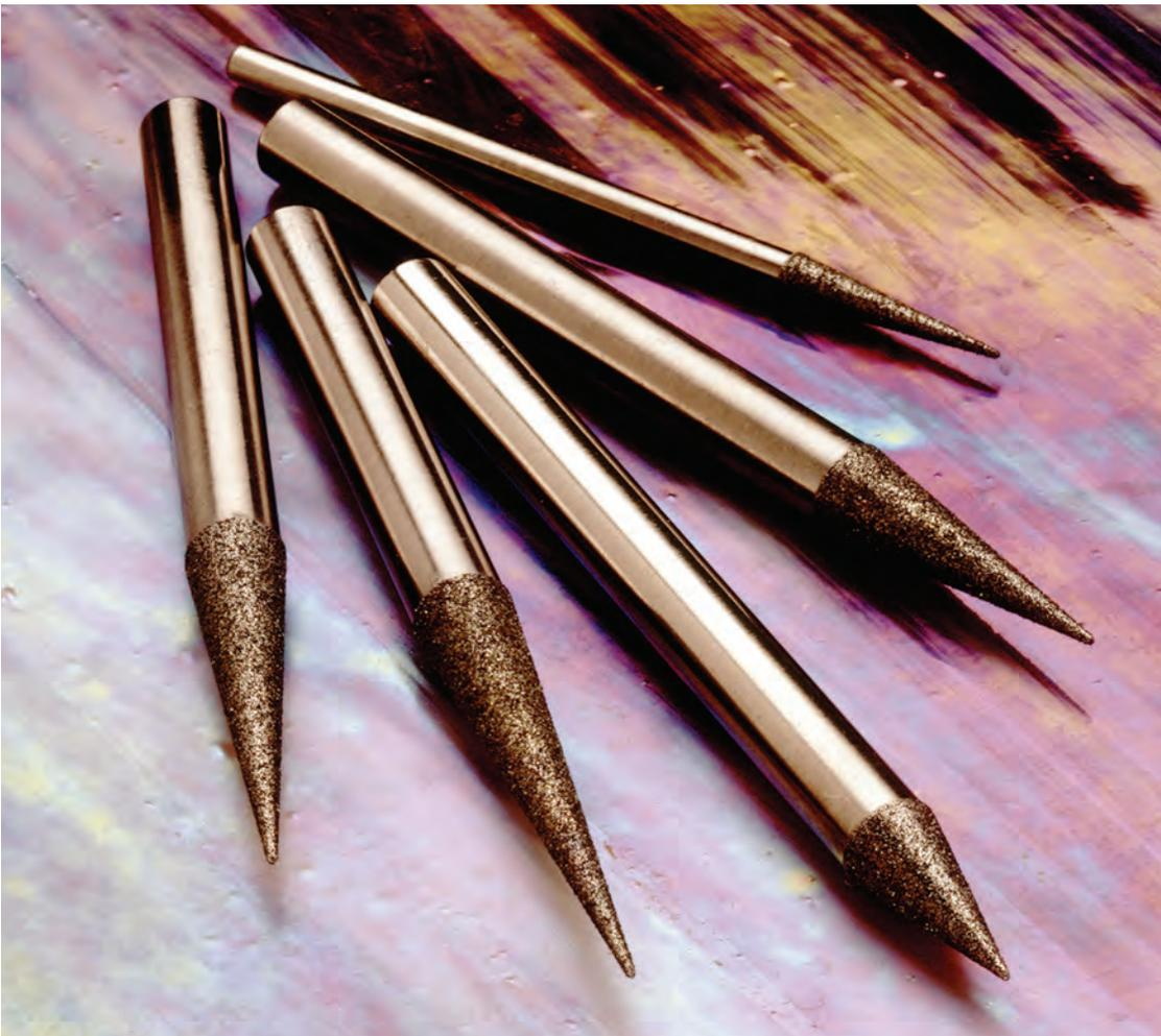
These diamond plated taper pins are ideal for grinding or ripping tungsten carbide drawing dies for the wire and tube industries and for cold heading dies. You get fast, efficient and precise grinding with long wear.
