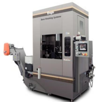
Specialty Custom Machines are designed to meet each customer's specific requirements. For example, in finishing Hammer Forged Rifle Barrels we included a precision reaming station for roughing followed by a series of 8 single-pass honing tools.
