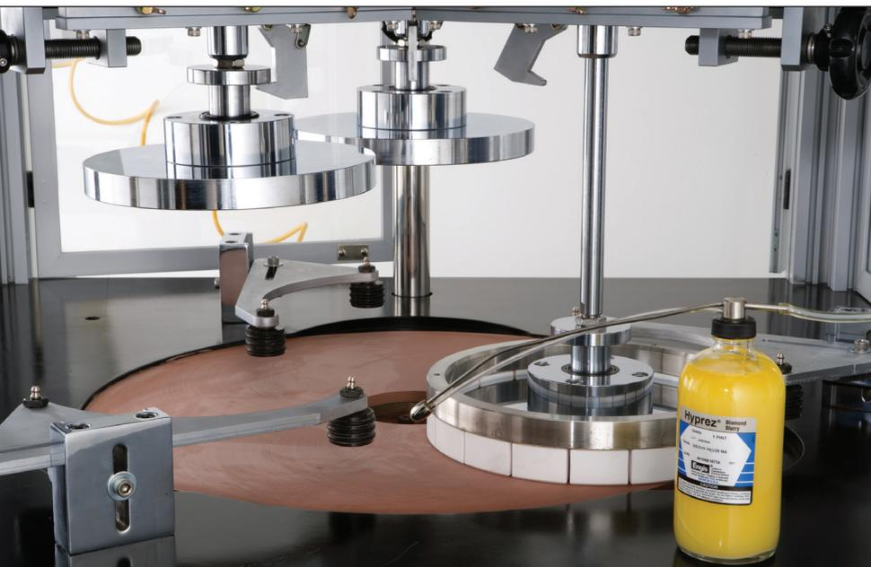
Lapping machines and precision lap plates are used to lap/polish ceramic parts and other stain-sensitive materials.
