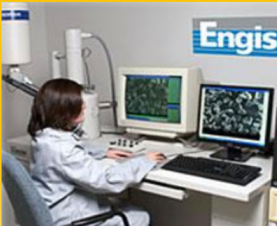
Scanning Electron Microscopy (SEM) provides qualitative data about diamond type, size and surface.
