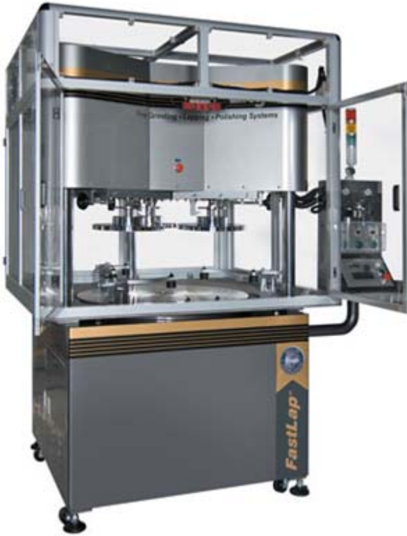
Model FL-42VP (Pneumatic) shown with optional Dust Cover & Hyprez Minimiser/Auto Dispensing System
